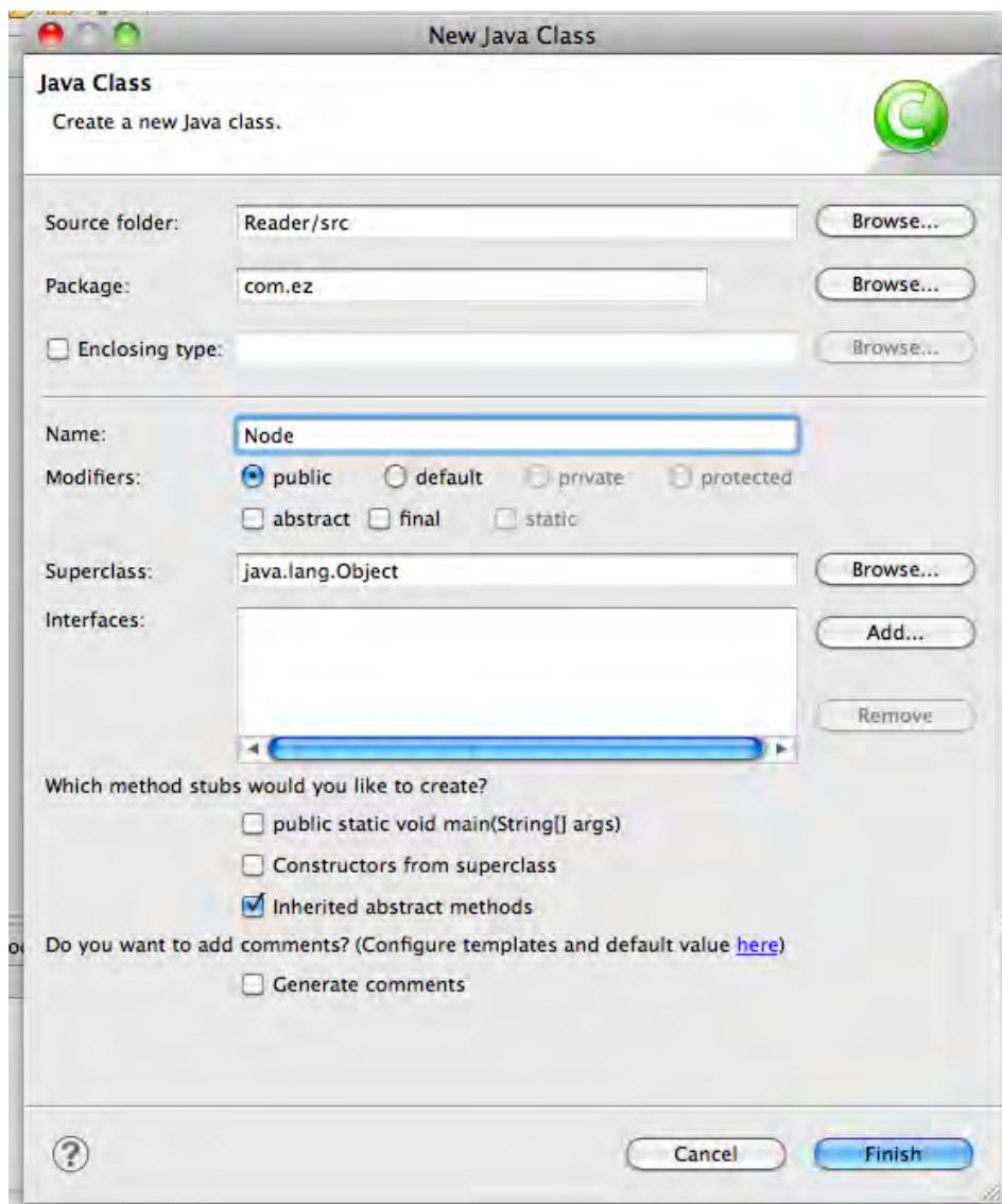
BECAUSE WE ARE GOING TO PASS NODE OBJECTS INTO THE DETAIL VIEW, WE NEED TO IMPLEMENT A “JAVA.IO.SERIALIZABLE” INTERFACE AND IMPLEMENT THE “SERIALVERSIONUID” PROPERTY (THIS IS A UNIQUE VALUE USED TO RECOGNIZE A SERIALIZED OBJECT; MOST IDES CAN GENERATE THIS FOR YOU, OR YOU CAN CREATE ONE YOURSELF):
