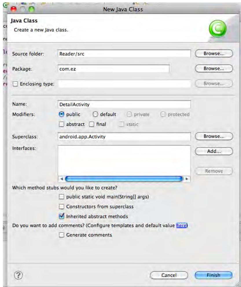
ONCE A NEW ACTIVITY CLASS IS CREATED, WE NEED TO REGISTER IT IN THE APPLICATION. IN ORDER TO DO SO, OPEN “ANDROIDMANIFEST.XML” AND PASTE THE FOLLOWING CODE BEFORE THE </APPLICATION> CLOSING TAG:
